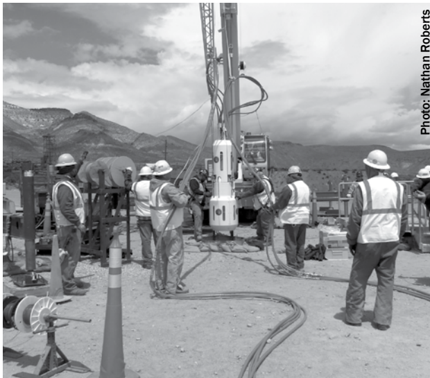
The SPE-4 Prime explosive canister is lowered into the borehole.
