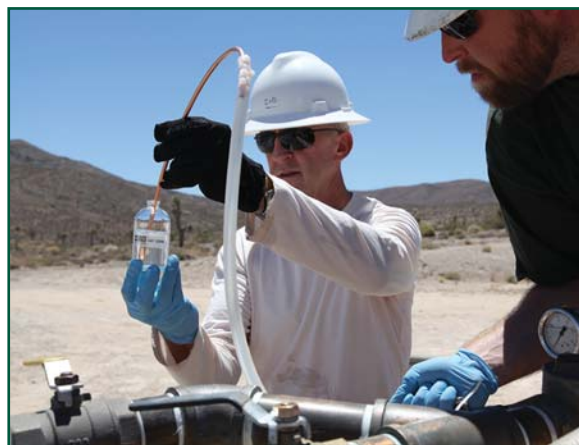
Hydrologists conduct water sampling at Well ER-6-2
