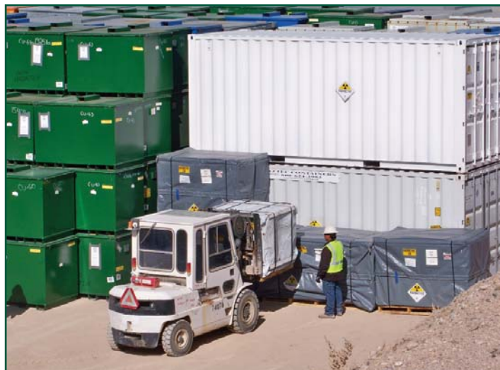
Waste packages are positioned in a disposal cell at the NNSA Area 5 Radioactive Waste Management Site
