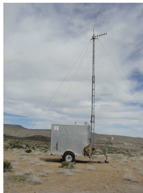
Figure A-12. Example of a typical MEDA station with a 10-meter tower
