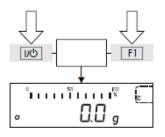
Upon completion of the automatic self-test, release the  $\boxed{\texttt{F1}}$  key as soon as the "C" is displayed (upper right corner of display).
