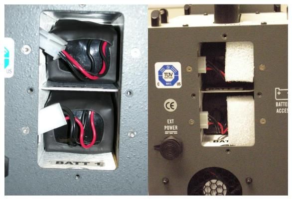
INCORRECT CORRECT Figure 6.8: Placement of Foam Spacers to Avoid Damage to Connector
