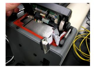
Figure 6.9: Access to the RS232 Port underneath the Display/Control Panel
