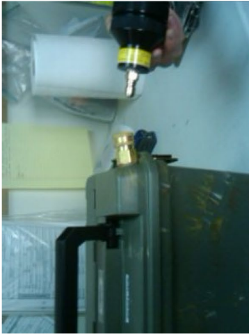
Insert the Sample Cassette assembly into the air sampler.
