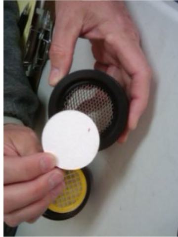
Install the paper filter fuzzy side out. If the front and back of the filter cannot be determined, then place an ink spot on the front of the filter near the edge. Record this in the comments on the Sample Control Form.
