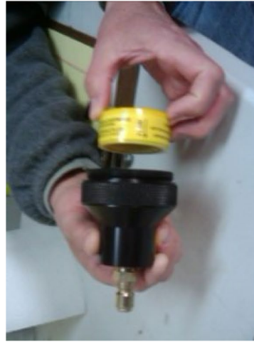
Install the cartridge. Ensure the Air Flow Arrow is pointing in the correct direction.
