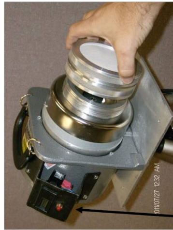
Attach the Sample Cassette to the Pump. Zero out the run time meter.
