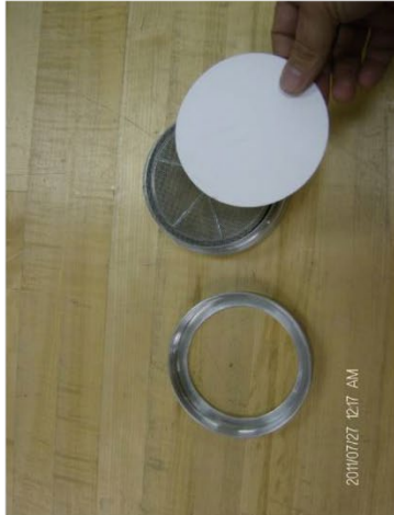
Install the paper filter fuzzy side out. If the front and back of filter cannot be determined, then place an ink spot on the front of the filter near the edge. Record this in the comments on the Sample Control Form.
