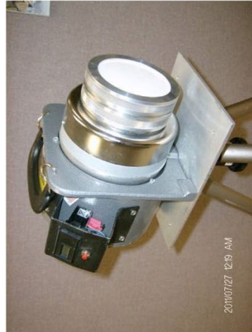
Air sample Cassette installed.
