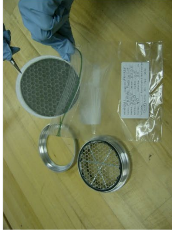
In a secure location, using tweezers, place the filter paper in a sample bag. Place a Security Seal on the bag.
