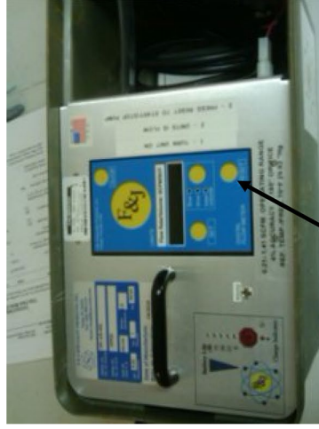
Press "RESET" to start Pump Wait till flow stabilized. Close the Lid.
