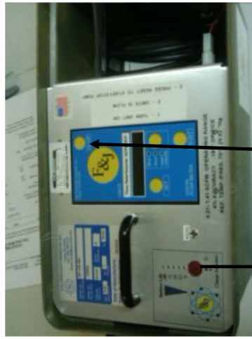
Insert the Sample Cassette assembly into the air sampler.
