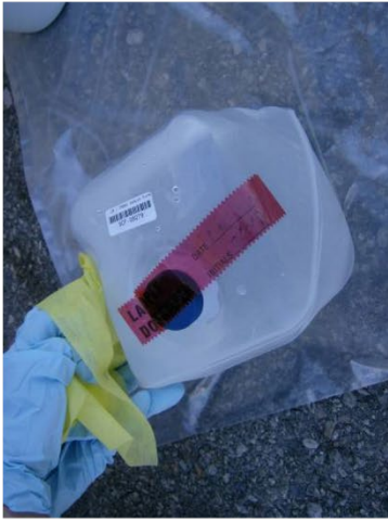
If needed, rinse the outside of the container with deionized or distilled water. Dry the outside of the sample container.
