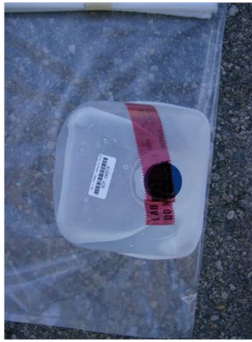
To prevent leaks, wrap tape around the lid and container (not shown in the picture). Place a Security Seal over the opening.
