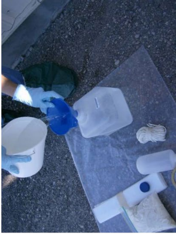
Using the funnel fill the 1 gallon (4 liter) sample container. Stop 1 inch from the top.
