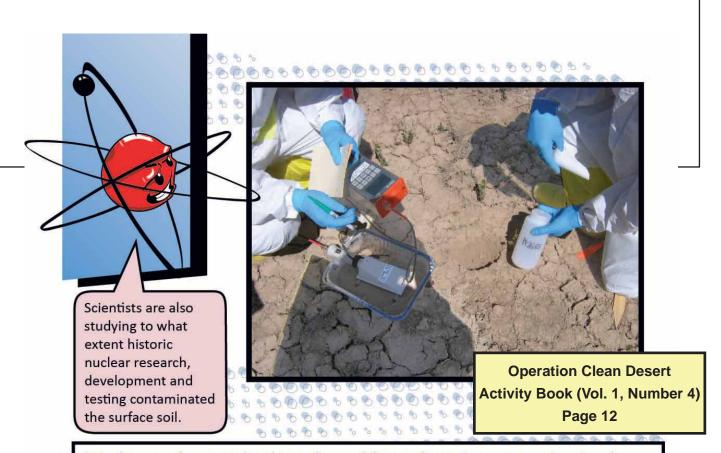
Workers today are checking the soil for radioactive contamination by using sophisticated hand-held instruments to conduct **radiation surveys** of the soil and by digging up, bottling and sending soil **samples** to special laboratories, where scientists then analyze the soil for various contaminants.
