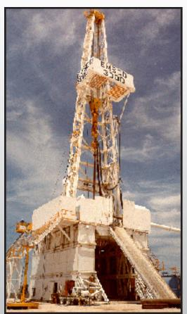
The EMSCO 3000, one of the largest drill rigs used at the NNSS.
