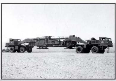
One of the 280 mm cannon's is shown completely assembled at Nellis Air Force Base on May 18, 1953, where it had just arrived by rail from Fort Sill, Oklahoma. Although it weighed 88 tons, its carriage was an ingenious foundation carried between two wheeled transporters, which were capable of speeds up to 40 miles per hour.
