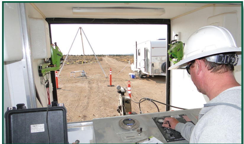
Bailer Sampling of Groundwater in Central Pahute Mesa
