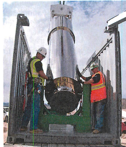
Figure 3 – During training, onsite workers remove a Type B shipping cask from the cargo container.
