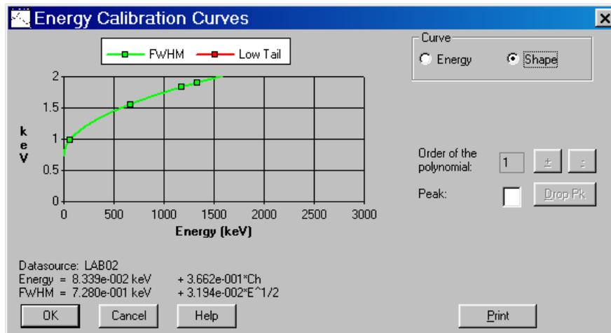
*Figure 6.7: Energy Calibration Curves Window Showing the Shape Curve*
