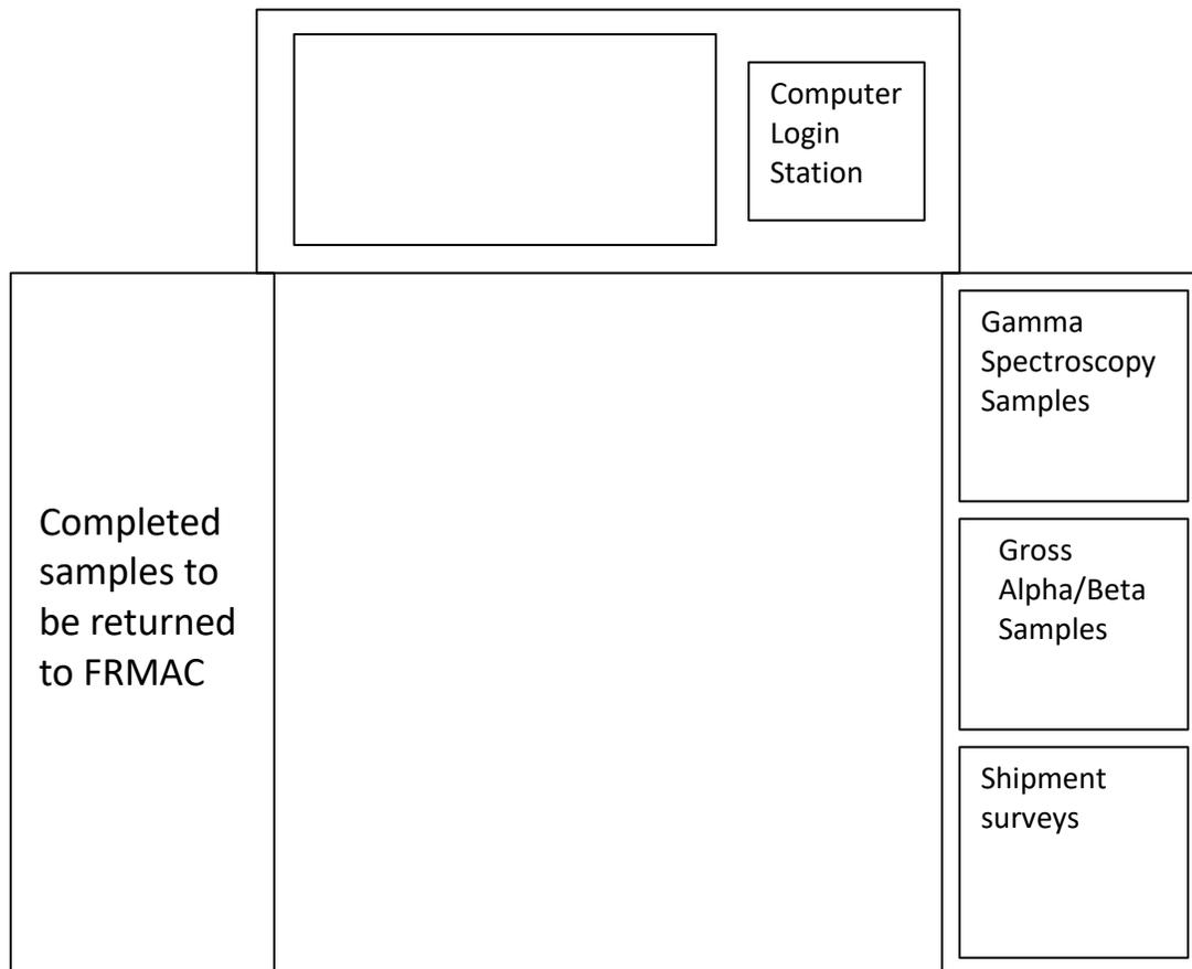
***Figure 4.1: Example - Sample Control Staging Area Recommended Setup***
