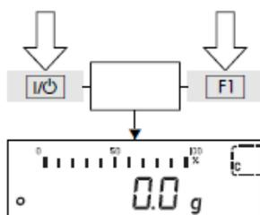
Upon completion of the automatic self-test, release the **F1** key as soon as the “C” is displayed (upper right corner of display).
