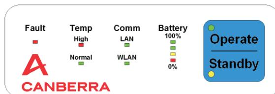
**Figure 6.2: FALCON 5000™ Control/Display Panel**
