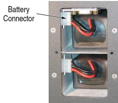
*Figure 6.3: FALCON 5000™ Battery ports and connectors*
