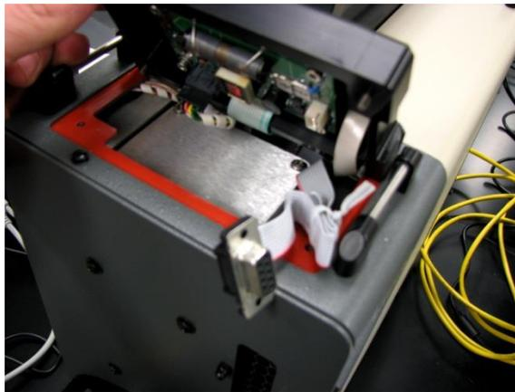
*Figure 6.9: Access to the RS232 Port underneath the Display/Control Panel*
