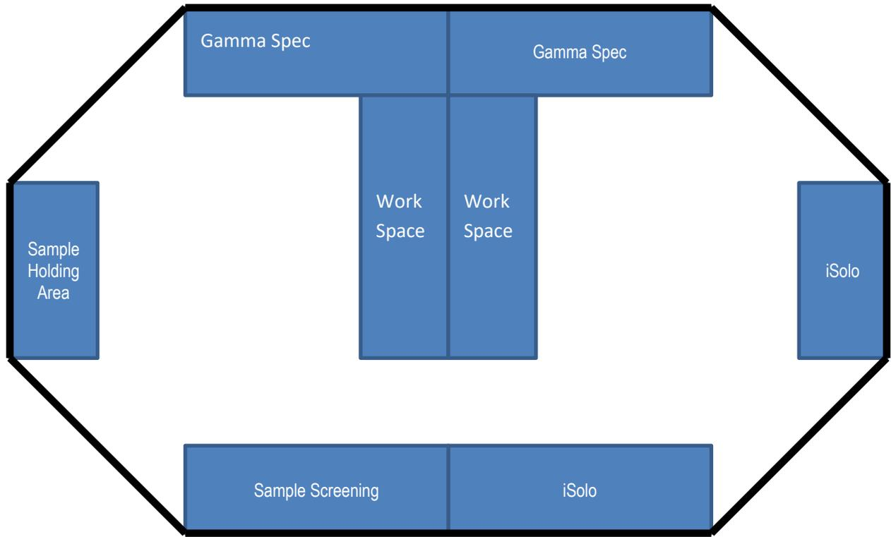
*Figure 5.1: Fly Away Laboratory Floor Diagram*
