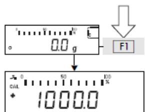
15. Center the 1,000 g calibration weight on the weighing pan, and then the balance self-calibrates automatically. The end of the calibration/adjustment is indicated by the weight unit symbol that appears on the display.
