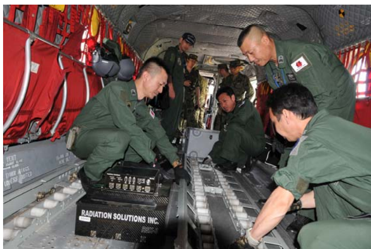
Figure 35. Japanese installing RSI equipment
