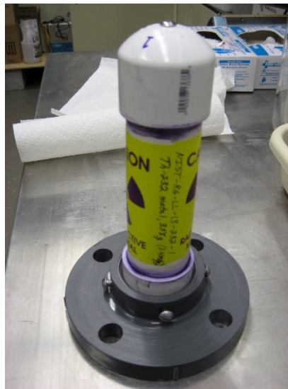
Figure 16-4. NIST traceable thorium bar source.
