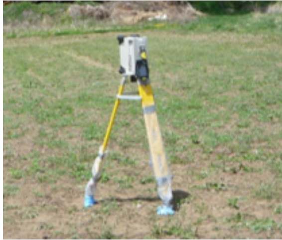
Figure 11-1. ORTEC Detective HPGe in-situ gamma spectroscopy measurement.
