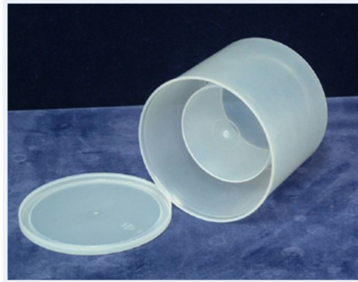
Figure 5-3. Photo of Marinelli container. [9]
