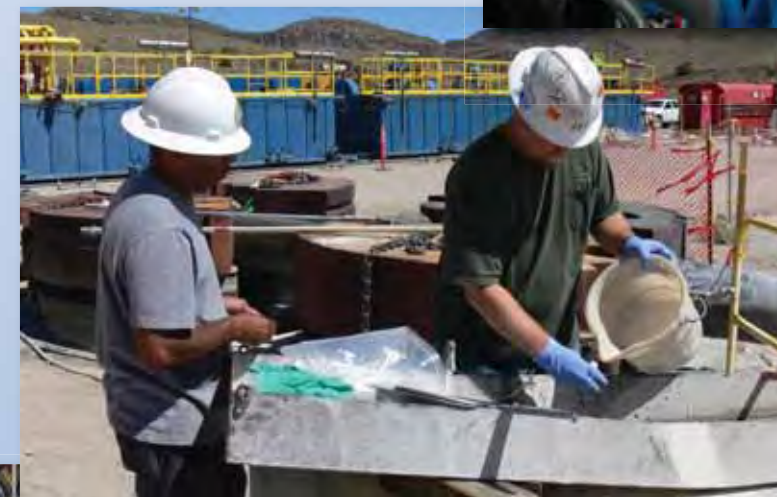
Groundwater characterization specialists collect drill cuttings from well drilling discharge fluids
