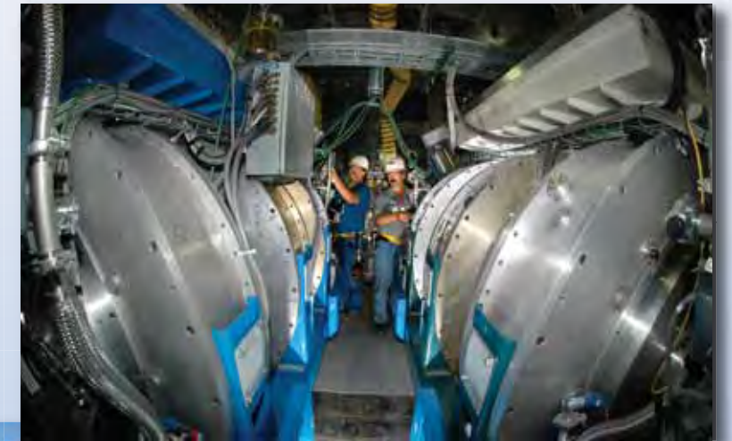
Cygnus (located in the U1a Complex) is a large X-ray machine used in subcritical experiments
