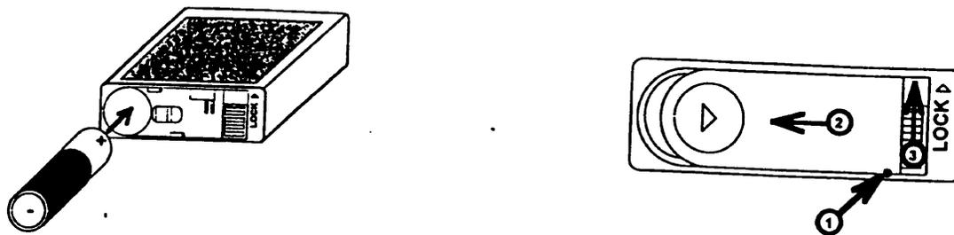
Figure I. Installation of AA battery in a PD-10i dosimeter
