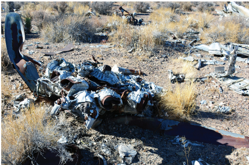
Skyraider drone crash including radial engine (DRI 2020)
