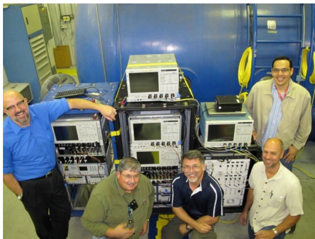
The MPDV team ( back row: M. Teel, A. Diaz; front row: C. Gallegos, C. Perez, E. Daykin ) pictured with the SDRD breakthrough multiplexed photonic Doppler velocimetry system. The MPDV has been used on experiments at Los Alamos National Laboratory as part of a broad collaboration with Lawrence Livermore National Laboratory and the Nevada National Security Site.
