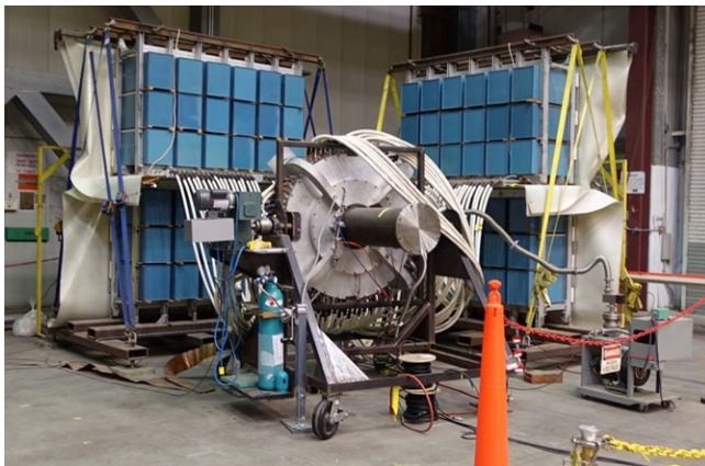
Dense Plasma Focus technology with a Marx system of two banks with 18 capacitors each
