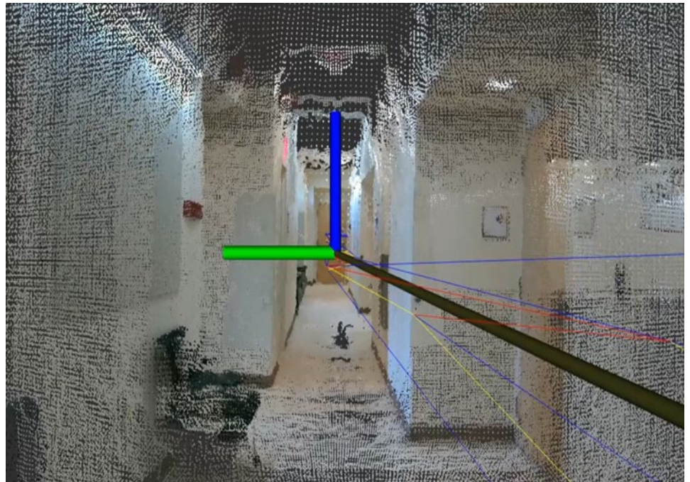
Simultaneous Localization and Mapping (SLAM) algorithm using an RGB-Depth camera to determine position of operator and sensor in XYZ space. The correlated XYZ and radiation detector measurements can be used to predict the location of a radiation source.
