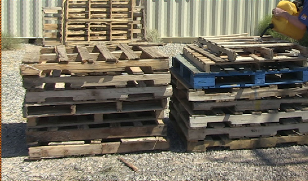
Upper left: dousing stack of pallets on right with diesel fuel; Lower right: dousing stack of pallets on left with F500 EA
