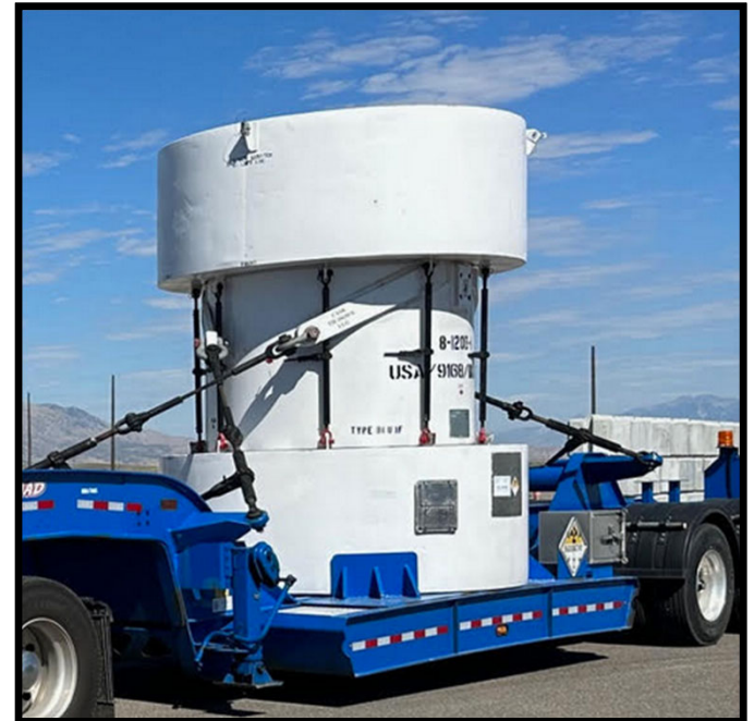
8-120B Cask holds (8) 55-gallon drums for transport from generator to the NNSS
