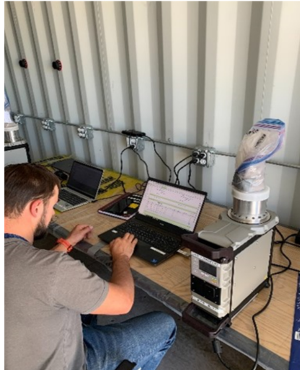
FAL staff analyze a ground deposition sample on an HPGe spectrometer.
