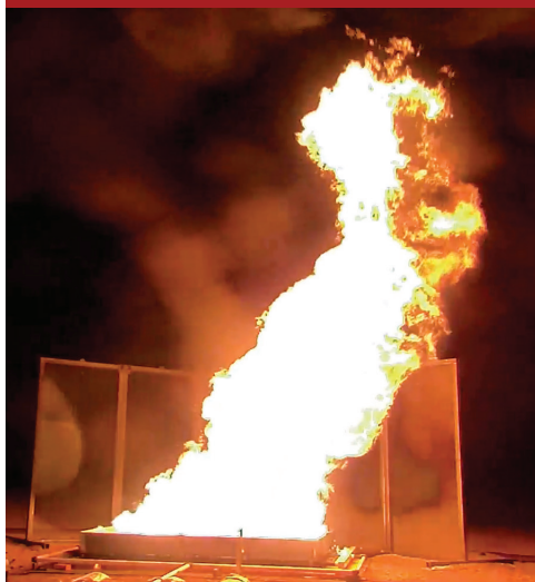
Fuel Fire experiment (mock test article) at BEEF.
