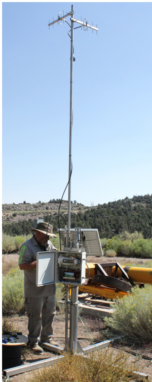
September 2024 node installation at U-12n.10 Vent Hole, a water level monitoring location for the Rainier Mesa/Shoshone Mountain CAU.
