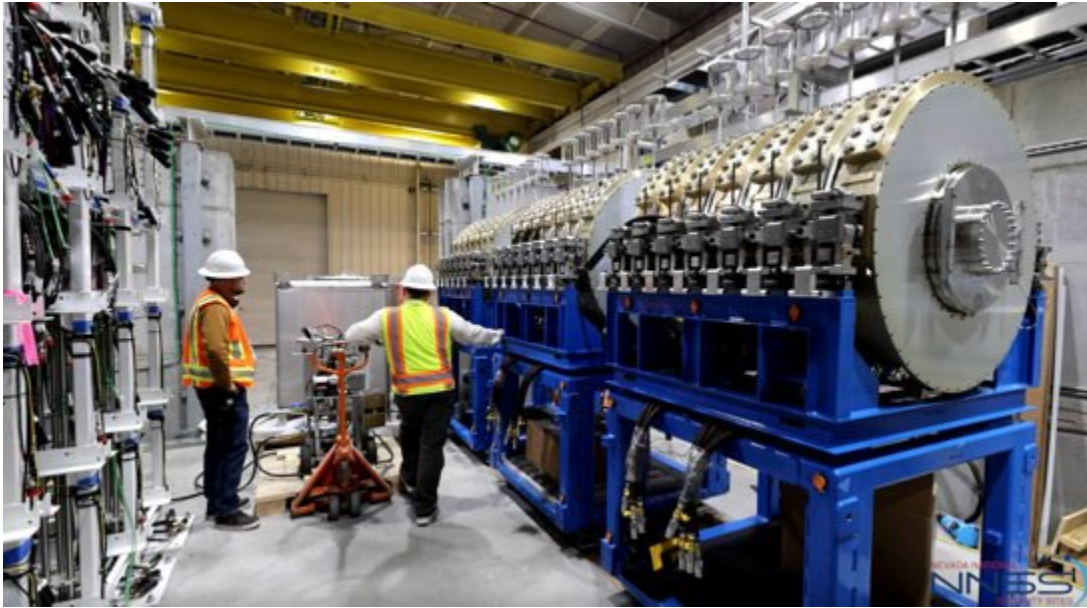
Figure 1. Scorpius modules installed at the Integrated Test Stand in North Las Vegas. Dr. Amber Guckes' FY25 feasibility study ("Combined Radiation Environment Modeling Using Scorpius," 25-170) explored the feasibility of using the Scorpius linear induction accelerator as a unique combined effects simulator.
